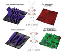
Ortho- or bay-tetracyanation? A comparative study on terrylenediimide reveals that the two functionalizations have similar impact on the optoelectronic properties, but remarkably different effects on selfassembling from solution, with striking consequences on the n-type behavior in field-effect transistors. The pronounced electron mobilities here reported for the bay-tetracyano derivative demonstrate the high potential of terrylenediimide as scaffold for n-type semiconductors.
