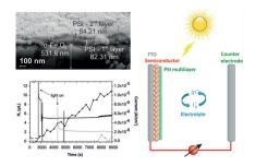
A fully integrated, stable, and functional photosystem I-based biohybrid dye-sensitized solar cell is constructed with an improved solar-to-electric quantum efficiency over previously reported biohybrid devices. A highly robust oriented Cyanidioschyzon merolae PSI-LHCI complex is used as a natural photosensitizer of the nanostructured hematite substrate for the sustained photodriven H<sub>2</sub> production.
