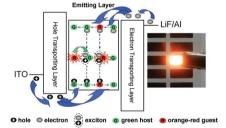
An all-phosphor host-guest doping system based on two novel Ir complexes possessing bipolar transporting ability realizes very-high efficiency orange-red phosphorescent organic light-emitting devices, which exhibit constant peak electroluminescent efficiency of >75 lm W<sup>-1</sup> for power efficiency and 26% for external quantum efficiency as well as extremely low efficiency roll-off within a range of 8 and 15 wt%.
