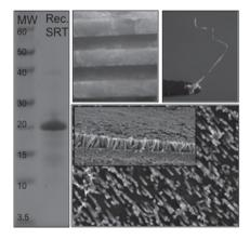
Protein sequences are identified in a squid ring teeth complex extracted from Loligo vulgaris and recombinant expression for its use in the fabrication of thermoplastic materials is demonstrated for the first time. Earlier attempts to create recombinant thermoplastic SRT protein failed due to the choice of larger molecular weight proteins. Reversible solid is demonstrated to melt phase transition of the recombinant protein, which is thermally shaped into any 3D geometries.
