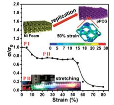
highly stretchable conductor manufactured by integrating porous poly(dimethylsiloxane) (p-PDMS) with a CNT/graphene network (pPCG). Mechanical simulation of p-PDMS demonstrates that large strains are accommodated through strut rotations and bending. After a slight decrease, the high conductivity (27 S m<sup>-1</sup> with 2 wt% CNTs/graphene) remained constant, even as the strain was increased to 50%.
