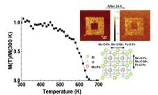
A new window for designing multiferroic materials through epitaxial strain control: For the first time, coexistent ferrimagnetism and ferroelectricity is demonstrated at RT in BiFe<sub>0.5</sub>Mn<sub>0.5</sub>O<sub>3</sub> (BFMO) by strain engineering. The most highly strained and crystalline films have a ferrimagnetic transition temperature of ≈600 K, which is 500 K higher than bulk BMO and a piezoresponse amplitude of 45 pm/V.
