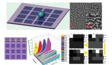
A self-powered, single-electrode-based tri**boelectric sensor** is reported to accurately detect the movement of an object/body in two dimensions. Based on the coupling of triboelectric effect and electrostatic induction, the motion information about the object, such as trajectory, velocity, and acceleration, is derived in conformity with the preset values.
