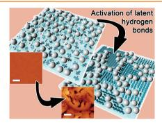
A new paradigm for the fine-tuning the phase segregation in SM-BHJs, based on the post-deposition exploitation of latent hydrogen bonds in binary molecular blends, is demonstrated. This approach allows fine-tuning of the nanoscale film connectivity and to simultaneously optimize charge generation and extraction via ordered phase-separated domains. As a result, the PV efficiency undergoes a 20-fold increase with respect to control devices.
